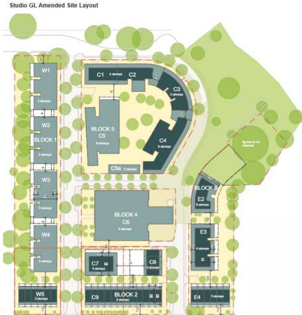
Figure 58 Revised site layout used to calculate amended FSR with changes requested by the Local Planning Panel
